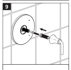
Re-install the nipple and stem extension and handle assembly.
