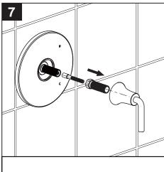
Remove the handle assembly and nipple and stem extensions.
