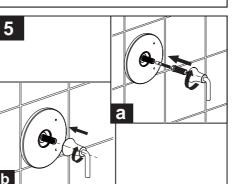
a.) Add the threaded nipple andpressure balance stem extensions.b.) Attach handle assembly.
