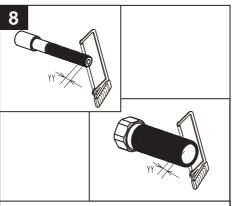
Cut stem and nipple extensions the amount noted in step # 6. (Never cut the stem and nipple while still on the valve. This may damage the valve.)
