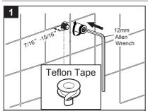
Apply teflon tape to supply nipple. Thread on supply nipple to 1/2" NPT water supply. Apply teflon tape to supply nipple and thread on bushing with 12mm allen wrench.
