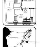
Position fill valve in tank, but do not fully install yet. Top of fill valve MUST be set 3" above overflow pipe. This will automatically place **CRITICAL LEVEL MARK / C.L. Mark**, 1" above the top of overflow pipe. Remove fill valve from tank to adjust height.
