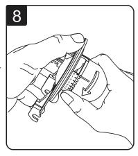
Remove the flapper from the flush valve by pulling up the frame of flapper one side at a time.
