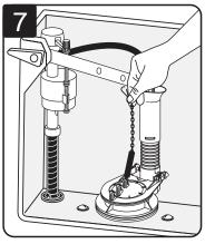
Connect the flapper chain to the tank lever. Allow for 1/2" of slack in the chain when the flapper is closed.
