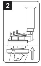
Slide new tank-to-bowl gasket over the nut with the narrow side facing down. Gasket should cover the nut completely.
