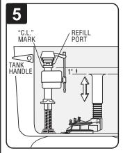
When installed, the top of the overflow pipe of the flush valve must be at least 1" below the C.L. mark of the fill valve.
