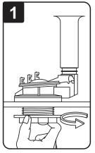
Before installing the flush valve in the tank, remove the tank-to-bowl gasket and nut from the bottom of the threads of the new flush valve. Position the overflow pipe toward the back of the tank but not over the bolt holes. Thread large nut onto the threads. Hand tighten only. DO NOT OVERTIGHTEN or tank may crack.
